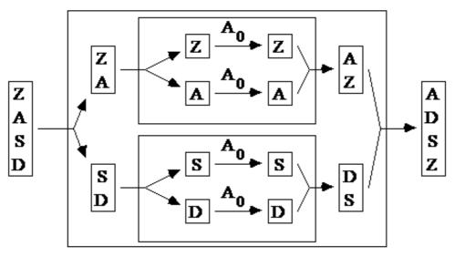
Exhibit 5.1: Sorting the sequence {Z, A, S, D} by using a divide-and-conquer scheme
