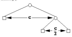
Exhibit 5.6: Sample layout obtained by halving horizontal displacement at each successive level
