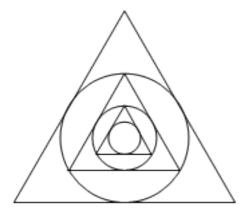
Exhibit 5.10: Interleaved circles and equilateral triangles cause the radius to be exactly halved at each step.
